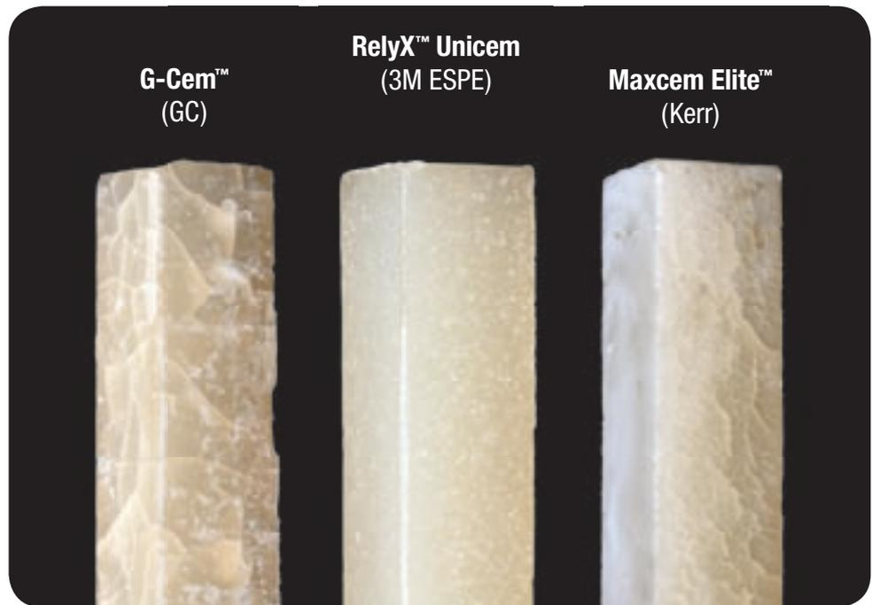
Results of thermocycling stress test on self-adhesive resin cements.
